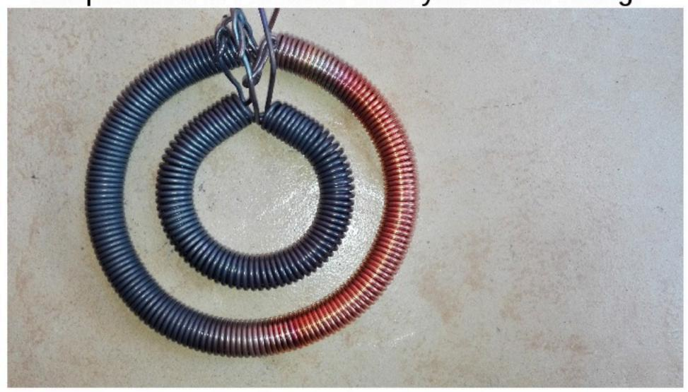
Ideal surface material is ceramic tile while doing this process. Never use metal surface, it will act as heatsink, resulting to inconsistent coating.
