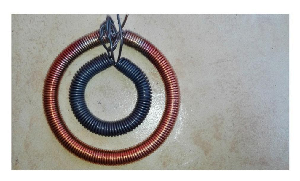
You'll get consistent bluish black color coating when you maintain a consistent temperature by movement speed. The tip of blue part of the flame should be touching the copper like a paint brush.
