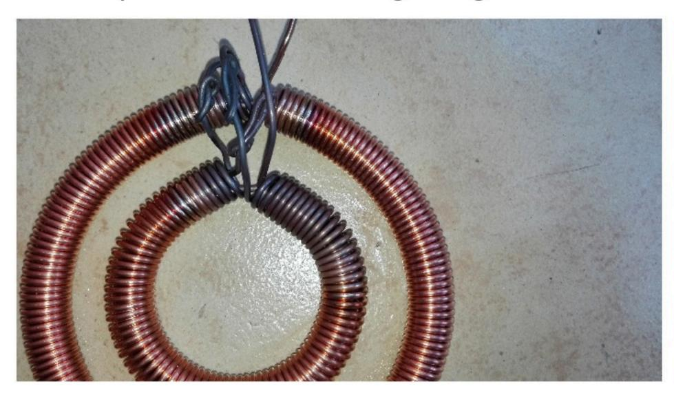
Move the flame up after completing the center loop and start moving counter clockwise around the outer loop.
