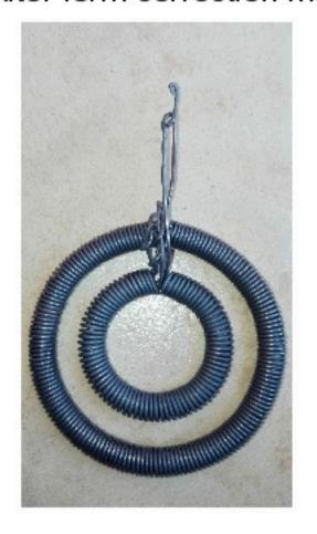
Form correction process can be done before a complete nano coating process. Simply preheat all at a lower temperature enough to align the copper material structure and let it cool for handling with gloves. Copper becomes softer after the heating process, one can make the desired shape then proceed to nano coating process.
