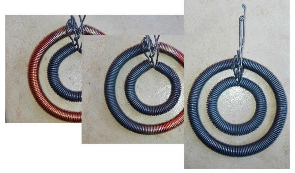
Start on the wire junction, temperature should be only be right before copper turns red hot.
