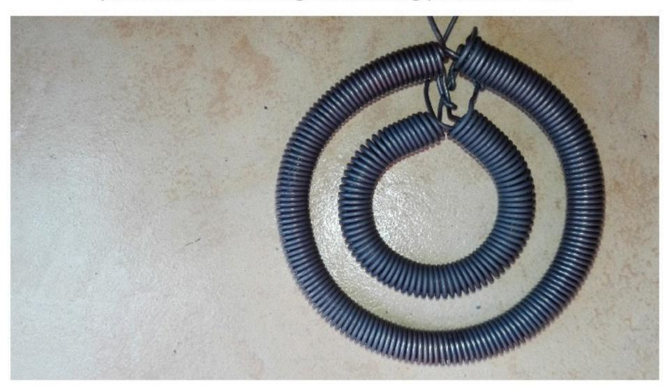
After cooled down by itself, one can make corrections on form then repeat the heating process one last time and it will be ready for use after cooling itself. Just leave it on the same tile while cooling.
