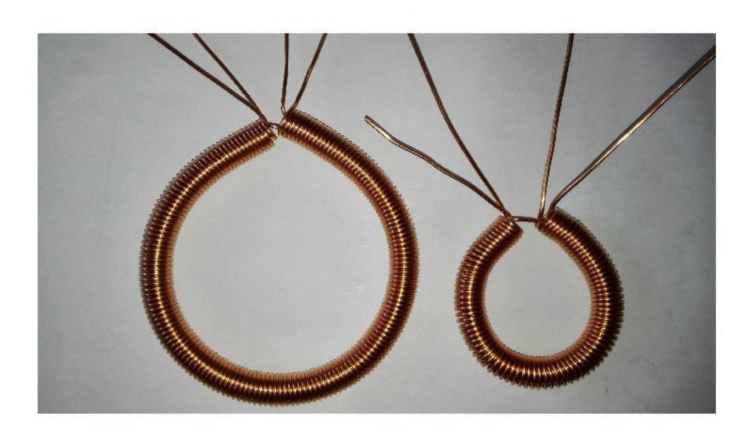
The smaller loop should be placed in the middle of the bigger loop before each individual wires.
