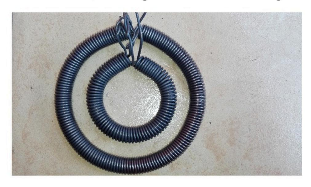
Do a similar process on the other side while still warm but of opposite direction on every loop to have a consistent flow of heat and nano material movement. An optional double flame opposite each other moving together while the coil is hanging on wire on its two terminals can do a single pass process both sides together, saving production time.
