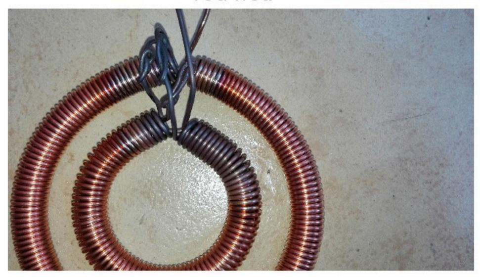
Move the flame towards the center loop and start moving clockwise slowly maintaining the desired temperature while moving along the coil.
